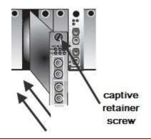
All open slots in the chassis must be covered with a face plate in order to maintain proper circulation throughout the chassis
