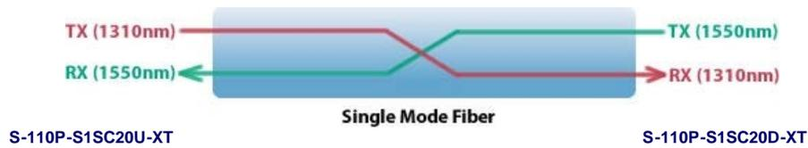
The majority of installations for single mode fiber media converters are of the “dual connector” or “dual fiber” type where one fiber connection is used for transmit, the other for receive. These are physically “crossed” to match up the Transmit/Receive links.
