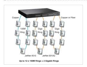
The JetNet 5728G-16P series supports the new generation ring technology – MSR<sup>TM</sup> which includes various new technologies for redundancy applications and structures of different networks. The PoE switch allows to aggregate up to 14 Rapid Super Rings, including 12 Fast Ethernet plus 2 gigabit Ethernet Rings. With the MSR<sup>TM</sup> technology, a node can be configured to multiple rings with the failover time in as little as 10ms, and zero-second of restoration time.
