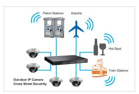
power mode (at 50°C) to outdoor PTZ IP cameras with direction control for cross–street monitoring, or WiMAX systems for internet access in train stations, airports or Hot-spots. The additional four Gigabit ports provide more resilient and redundancy for users while forming ring networks and delivering increased bandwidth to the central network.
