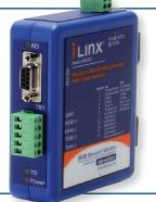
Model BB-485DRCi industrial-grade isolated serial converter changes RS-232 signals to RS-422 for increased range, or to RS-485 for increased range plus multi-drop capability.
