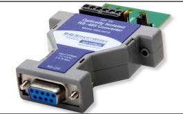
Model BB-485OI9TB, isolated converter, converts unbalanced, full-duplex RS-232 signals to balanced full-duplex (4-wire) RS-422/485 or half-duplex (2-wire) RS-485 signals.
