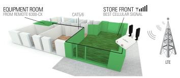
Site survey using the included battery will help you locate the best signal strength to send back to your router while remotely powering using the included PoE injector.
