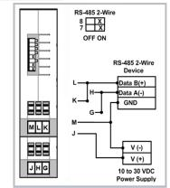
Jump L to K and H to G and power the 485OPDR. Set dip switches to RS-422 or RS-485, depending upon what you are using to connect to the PC. Set the baud rate to 9600.
