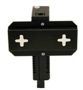
The IE-MultiWay can be mounted with two DIN Rail clips, a hardware option available through IMC Networks. The DIN Rail clips include screws, to allow the installation onto a DIN Rail. Install the screws into DIN Rail clips, which can be mounted parallel or perpendicular to the DIN Rail. Snap the converter onto the clips. To remove the converter from the DIN Rail, use a flat-head screwdriver into the slot to gently pry the converter from the rail. Refer to picture on page 7.
