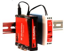
IE-MultiWay with optional DIN Rail mount power supply
