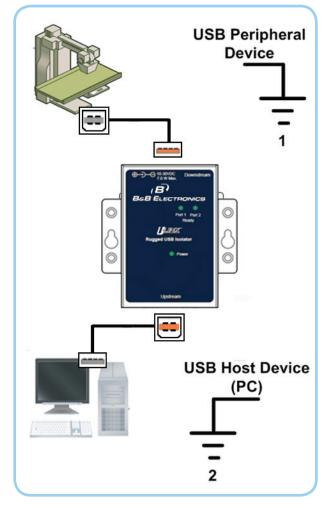
For optimum isolation the computer/host and the connected device should not use the same ground.
