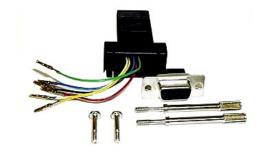
Model# BB-9F8CK modular jack adapter features a DB9 male connector, an RJ45 female connector and eight wire leads. Used for modular RS-232 connections, the adapter converts DB9 female serial connections to RJ45 female connections (phone jack, network jack). The BB-9F8CK also allows customized serial pin-out configurations.
