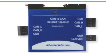
Model BB-CANOP increases the node capacity of CAN (Control Area Network) systems while protecting CAN networks from component destroying surges and transients. The BB-CANOP provides 2,000 VDC of optical isolation to separate and protect critical segments of the system from the rest of the CAN Network. It is protocol independent, allowing it to work with different CAN protocols and frame lengths.
