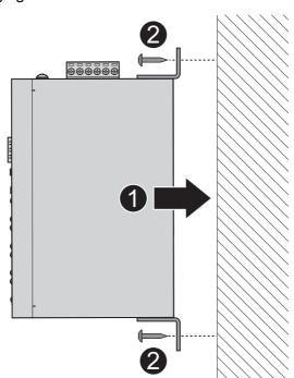
**Figure 2.11 Wall Mount Installation**
