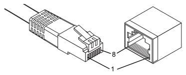
Figure 2.17 Ethernet Plug & Connector Pin Position
