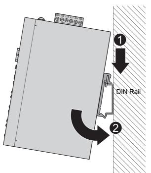
Figure 2.7 Installing the DIN-Rail Mounting Kit
