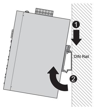
Figure 2.8 Removing the DIN-Rail
