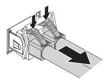
Figure 2.15 Removing a Fiber Optic Cable to a Transceiver
