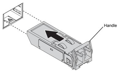
Figure 2.13 Installing an SFP Transceiver
