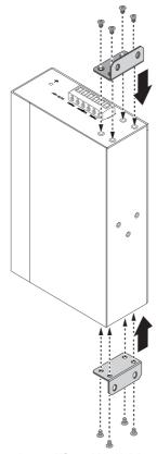
Figure 2.9 Installing Wall Mount Plates
