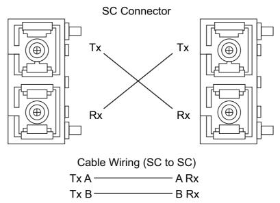
Figure 2.18 Pin Assignment of the SC Connector
