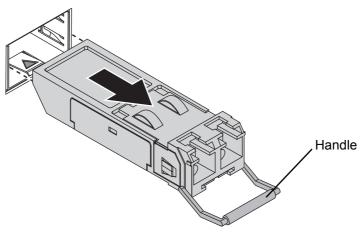
Figure 2.16 Removing an SFP Transceiver
