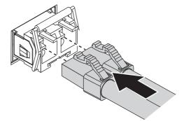
Figure 2.14 Attaching a Fiber Optic Cable to a Transceiver
