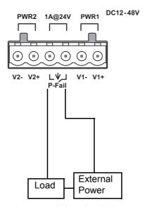
Figure 2.19 Power Wiring for EKI-2741FI/LXI/SXI
