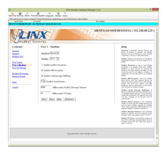
Figure 32. Modbus Port Screen
