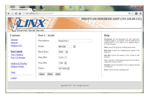
Figure 47. Serial Port 1 Setup
