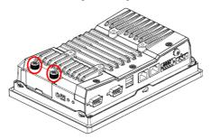
Insert the CFast or SD card into the slot using the push-push mechanism.
