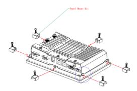
Use a torque of 4Kgf-cm to secure the mounting screws to fasten the panel-mounting kit onto the wall.
