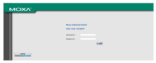
**NOTE** By default, the password assigned to the Moxa switch is **moxa**. Be sure to change the default password after you first log in to help keep your system secure.
