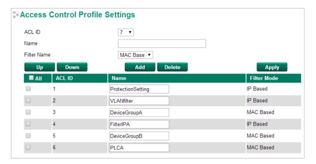
On this page, you can configure two settings: (1) Add/Modify Access Control list, and (2) Adjust ACL ID.
