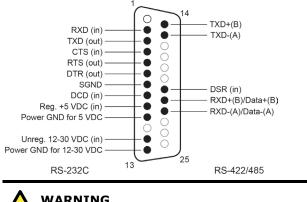
Pin 1 is reserved for debugging. Connecting this pin yourself could result in irreparable damage to your device.
