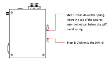
To remove the NPort IAW5x50A-6I/O from the DIN rail, reverse Steps 1 and 2.
