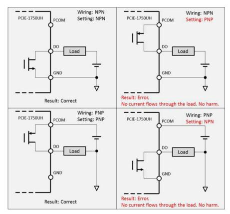
Figure 3.6 Wrong connection wouldn't damage the IDO component
