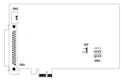
Figure 3.1 Card layout of PCIE-1750U/UH
