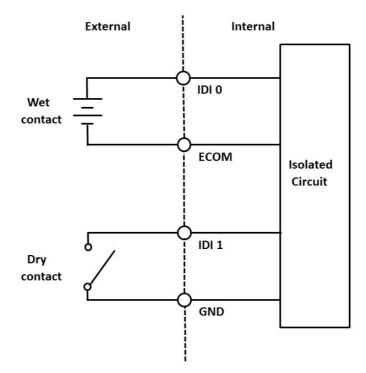
Figure 3.3 Isolated DI Connection
