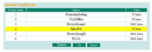
Changing an established access control list's priority is easy. Moxa provides a simple interface to let you easily adjust priority. Follow the three steps below to adjust the priority:
