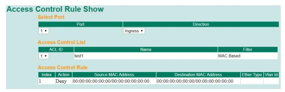
NOTE For TN-5800A series, there are two limitations on ACL settings. Based on the ingress port type of ACL rules, there are two types for the limitation of numbers.
