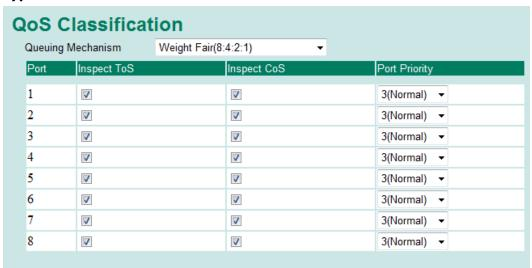
The Moxa switch supports inspection of layer 3 TOS and/or layer 2 CoS tag information to determine how to classify traffic packets.
