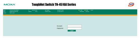
**NOTE** By default, the password assigned to the Moxa switch is moxa. Be sure to change the default password after you first log in to help keep your system secure.
