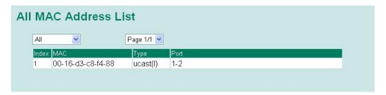
The MAC Address table can be configured to display the following Moxa switch MAC address groups, which are selected from the drop-down list:
