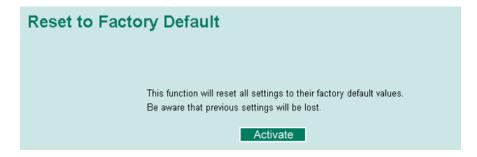
This function provides users with a quick way of restoring the Moxa switch's configuration to factory defaults. The function is available in the serial, Telnet, and web consoles.
