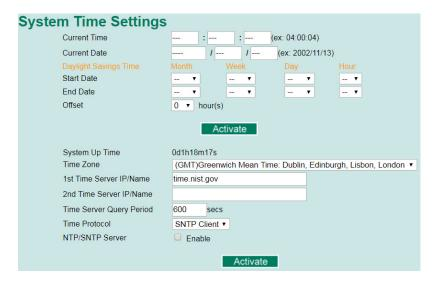
The Moxa switch has a time calibration function based on information from an NTP server or user specified time and date. Functions such as automatic warning emails can therefore include time and date stamp.
