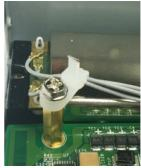
18. Plug the antenna onto the connector.
