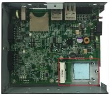
Remove the screw next to the socket and replace it with the bronze screw (in the package) as shown below:
