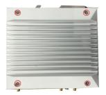
5. Remove the three screws on the top panel.
