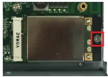
14. Connect antenna cables to the cellular module. There are three antenna connectors on the cellular module: W1 and W3 are for cellular antennas and W2 is for GPS antenna.
