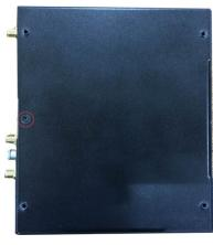
6. Remove the two screws on the bottom panel.
