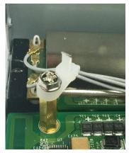
18. Plug the antenna onto the connector.
