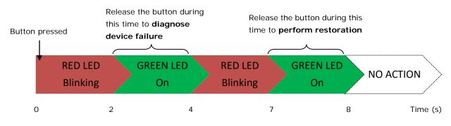
The LED indicators behave differently when diagnosing a device failure compared to performing a firmware restoration. See the following table for details:
