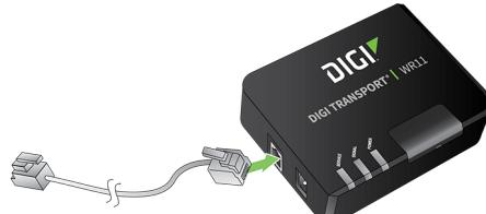
**Note** Position the Digi TransPort WR11 on a flat, level surface in a location with adequate ventilation. The unit is designed for indoor use. **Do not expose the unit to extreme heat or cold, strong magnetic fields, or liquids.**
