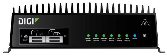
Press and hold the **Reset** button for **15** seconds. The device reboots automatically.
