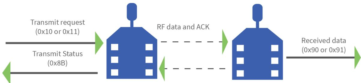
The device sends the 0x8B Transmit Status frame at the end of a data transmission unless you set the frame ID to 0 in the transmit request. If the packet cannot be delivered to the destination, the 0x8B Transmit Status frame indicates the cause of failure.
