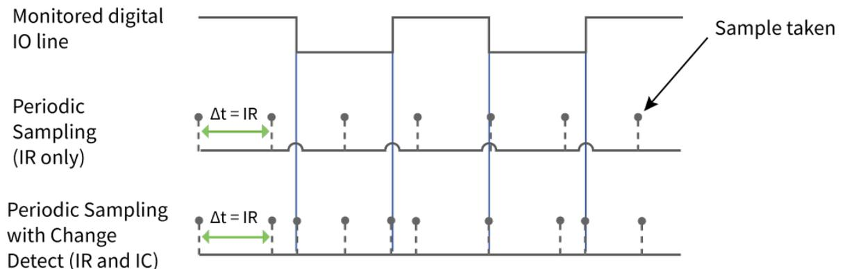
**Note** Use caution when combining Change Detect sampling with sleep modes. **IC** only causes a sample to be generated if the change takes place during a wake period. If the device is sleeping when the digital input transition occurs, then no change is detected and an I/O sample is not generated. Use **IR** in conjunction with **IC** in this instance, since **IR** generates an I/O sample upon wakeup and ensures that the change is properly observed.
