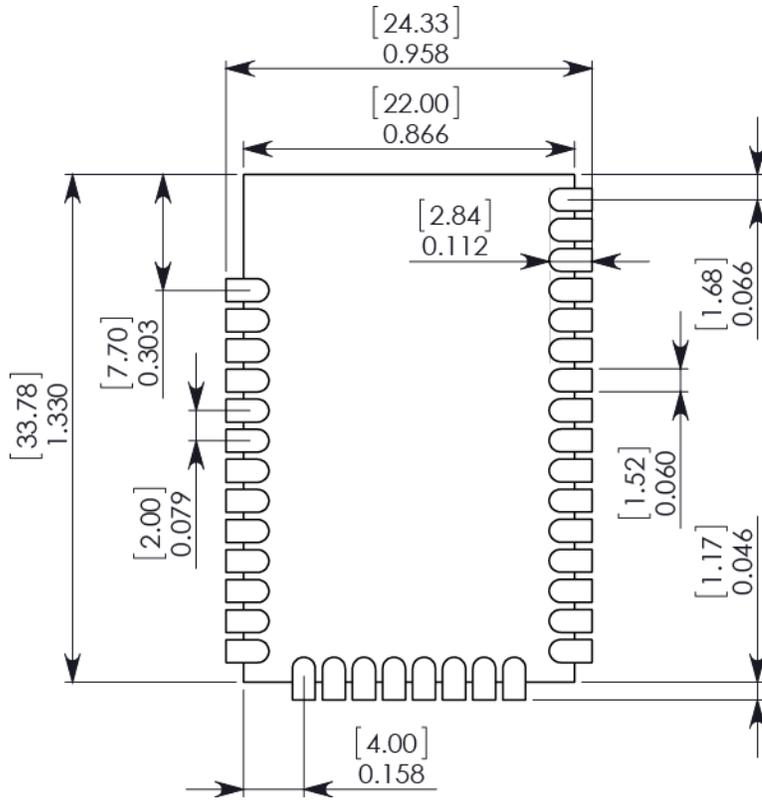
Match the solder footprint to the copper pads, but you may need to adjust it depending on the specific needs of assembly and product standards. We recommend a stencil thickness of 0.15 mm (0.005 in). Place the component last and set the placement speed to the slowest setting.
