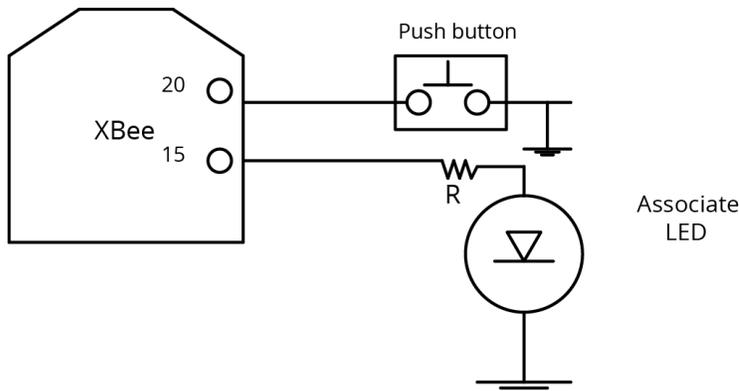
To support the Commissioning Pushbutton and its associated LED functions, connect a pushbutton and an LED to device pins 20 and 15 respectively.
