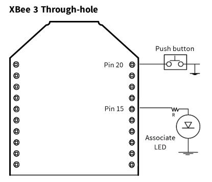
A pushbutton and an LED can be connected to the through-hole-mount device to support the commissioning pushbutton and associate LED functionalities.
