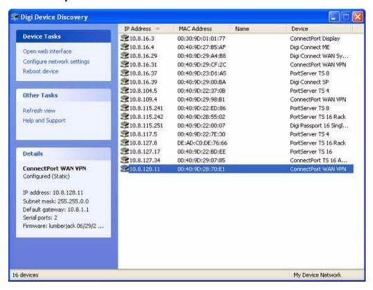
3. Depending on whether a system administrator has configured password authentication for the device, a login may be required. If a login dialog is displayed, enter the user name and password for the ConnectPort LTS product. The default username is **root** and the default password is **dbps**. If these defaults do not work, contact the system administrator who initially set up the device.
