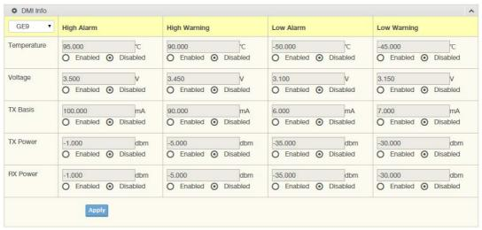
Figure 116: Diagnostics > DDM > Diagnostic Alarm Information
