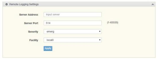
Figure 114: Diagnostics > System Log > System Log Server
