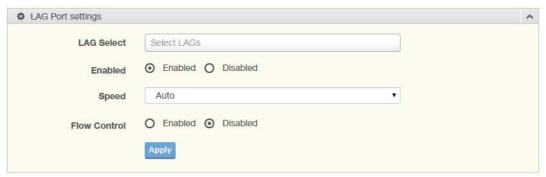
Figure 49: L2 Switching > Link Aggregation > LAG Port Settings
