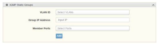
Figure 61: L2 Switching > Multicast > IGMP Snooping > IGMP Static Groups
