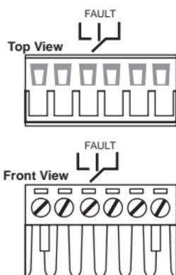
**FAULT:** The two middle contacts of the 6-contact terminal block connector are used to detect both power faults and port faults. The two wires attached to the Fault contacts form an open circuit when:
