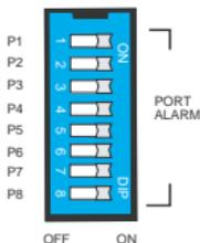
The default setting for each DIP switch is OFF. The following table explains the effect of setting the DIP switches to the ON positions.
