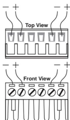
**STEP 1:** Insert the negative/positive AC/DC wires into the V-/V+ terminals.
