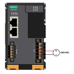
**NOTE** The 12/24 VDC field power supply can be connected directly to 45MR modules. If more connection points are needed, purchase 45MR-7820 (8 x FP+ and 8 x FP-) modules.
