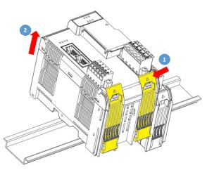
**NOTE** Disconnect all connections, including Ethernet, serial, and power cables, from the device before removing the device from the DIN rail.
