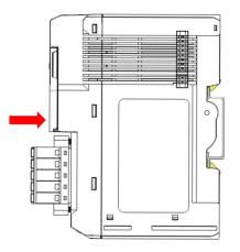
**INFORMATION** When the I/O module is inserted into the correct position, the connection between the internal bus and the previous module is established.
