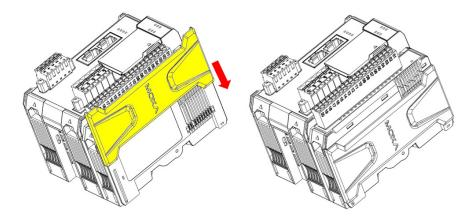
**NOTE** The covers provide protection against electrostatic discharge.
