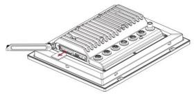
3. Reattach the cover and secure it with screws.
