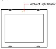
The ambient light sensor helps automatically adjust the brightness of the panel with the ambient light condition. This function is disabled by default and has to be enabled before it can be used. For details, refer to the MPC-2121 Hardware User's Manual.
