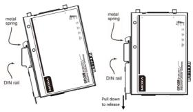
To remove the OnCell 3120-LTE-1 from the DIN rail, pull down the lever at the bottom of the DIN-rail kit.
