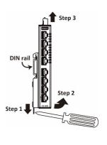
**NOTE** Screws that are used to fix the DIN-rail kit on the SDS-3016 should be securely fastened before mounting on the mounting rail. Please make sure that if you remove the DIN-rail, it must be securely fastened when it is reattached.
