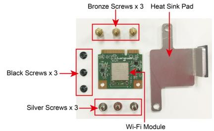
Follow these steps to install the Wi-Fi module for the UC-8220 Series.
