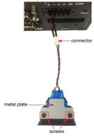
Separate the connector and remove the two screws on the metal plate.
