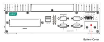
2. Unfasten the two screws on the battery cover.
