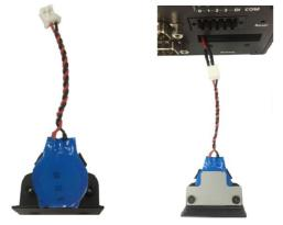
Reconnect the connector, place the battery holder into the slot, and secure the cover of the slot by fastening the two screws on the cover
