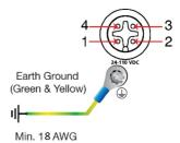
The power input specification is given below:
