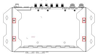
The four screws for the mounting brackets are included in the product package. They are standard IMS $\_$ M3x5L screws and require a torque of 4.5 kgf-cm. Refer to the following illustration for details.
