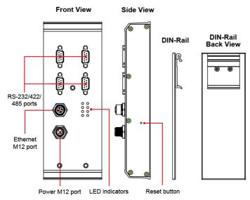
The Reset to Default Button—Press the reset button to default button for five seconds continuously to load the factory default settings. Use a pointed object, such as a straightened paper clip or toothpick, to press the reset button to default button. This will cause the Ready LED to blink on and off. The factory default settings are loaded once the Ready LED stops blinking (after about five seconds). At this point, you can release the reset button to default button.
