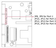
Jumpers are used to set the pull up/down resistors. The default is 150 K $\Omega$ . Short the jumpers to set this value to 1 K $\Omega$ . Do not use the K $\Omega$  setting with RS-232 mode, since doing so will degrade the RS-232 signals and shorten the communication distance.
