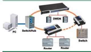
NPort 6000 series supports the Turbo Ring function for the cascade topology. With Turbo Ring, if any segment of the daisy chain ring becomes disconnected, the network will recover in less than 300 ms.
