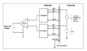
Figure 3-3: Differential input channel connection - ground reference signal source
