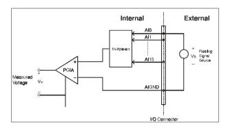
Figure 3-2: Single-ended input channel connection
