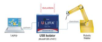
The USB isolator is transparent to the operating system. It will not appear in the device manager. Operation of the isolator can be verified by the "Power" ON LED. This indicator illuminates when the device is plugged in to a 500 mA port.
