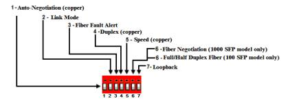
Note: All switch changes take effect immediately and will result in a link reset on both ports.
