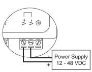
The TCC-120/120I is powered by an external 12-48 VDC power supply. To connect to the power supply, run two wires from the V+ and V- terminals, on the TCC-120's 3-connector terminal block, to the DC power supply, as shown in the figure on the left.
