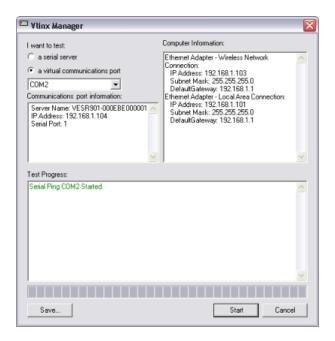
Figure 42. Testing a VCOM Port
