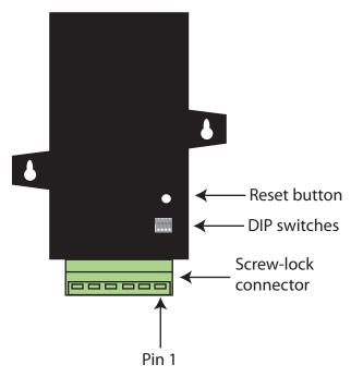
The adapter is switch-selectable between RS-422 half duplex/full duplex, and RS-485 modes (see DIP switches on page 26). The function for several pins varies between RS-422 and RS-485 modes.
