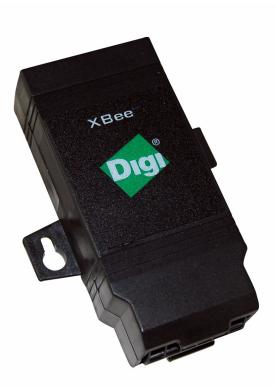
The XBee Sensor Adapter provides short-range wireless connectivity to Digi Watchport<sup>®</sup> Sensors. Unlike an embedded wireless module, which requires design integration and development time, these off-the-shelf adapters provide instant wireless connectivity to existing Watchport Sensors. All XBee adapters can be used with Digi's gateways for data aggregation and IP connectivity.
