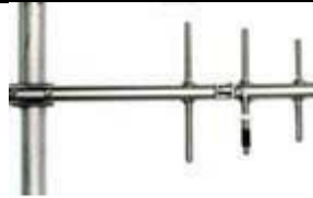
Figure 3-12 Representative Yagi Antenna
