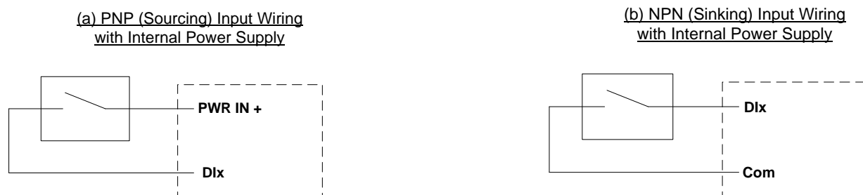
Figure 4-3 Typical Digital Input Wiring for PNP and NPN connection types (with internal PS)
